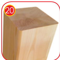
20 Soft conifer wood 140 x 140 mm, coreless, knotless, glued in layers with polyurethane glues, totally resistant to water. Wood secured from weather conditions in the process of impregnation carried out twice with specialist wood protecting impregnating preparations.
