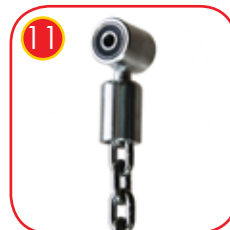
11 Swing slings, with double bearings, made of stainless steel guarantees a quiet mechanism operation. Beside the horizontal movement it allows as well for the circular movement to avoid twisting of the chain.
